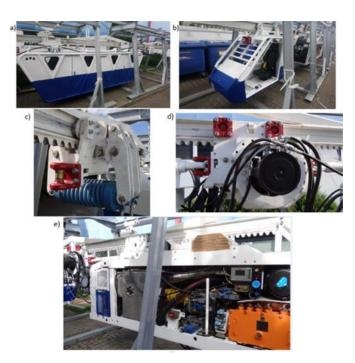
Fig. 2. Components of the suspended monorail on the testing track: a) personnel cabin, b) operator's cabin, c) breaking trolley, d) gear drive with built-in multi-disk brake, e) machinery part [7]
